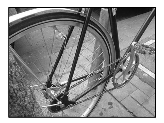
Pushing on the pedals makes a big gear turn. The big gear makes a chain move. The chain makes a small gear turn. That small gear makes the bike's back wheel turn, and the wheel pushes on the road to make you move.
