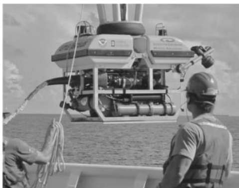
This deep sea robot named Little Hercules can explore up to 4,000 meters below the surface of the ocean. This picture shows the robot being lowered into the ocean for a test drive near Hawaii.
